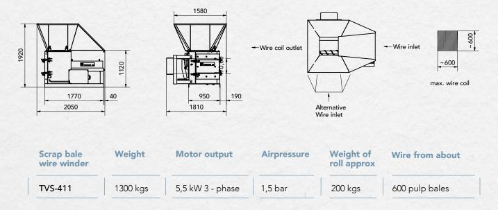
The scrap wire bundling machine TVS-411 has a heavy steel structure design and need no fixing bolts. The machine is provided with geared motor, necessary electric equipment and safety device with limit switches. It is delivered completely assembled and tested in our workshops. Easy to connect and start operation.
