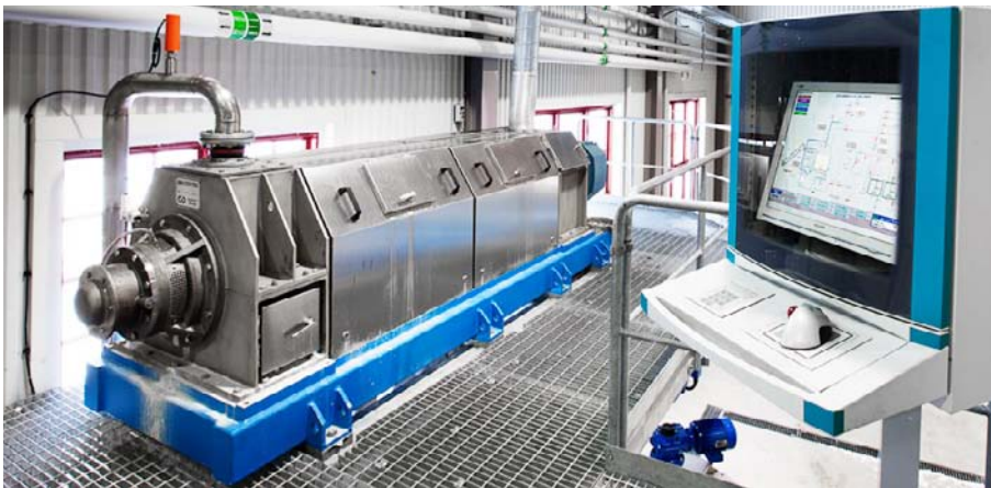
Thickening by screw press.
