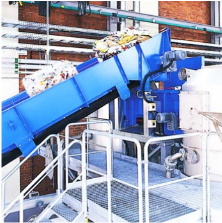
Feeding waste paper or pulp to LC-, MC-, or HC pulper.
