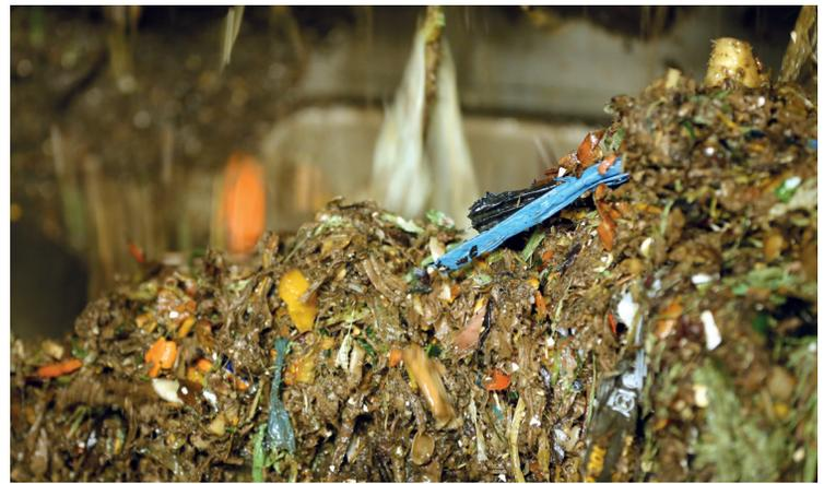
Separated contaminants consisting mainly of plastic- and carton packaging along with citrus peels coming out of the reject separator before going into the dewatering process. Notable is the intact "unmacerated" condition.
