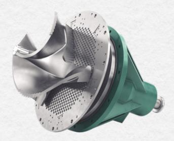
The hydrodynamic design of the vanes provides a combined handling of the pulp. On the front side of the vane the pulp pressure is down towards the screen plate and the dissolved pulp gets forced out through the strainer holes.
