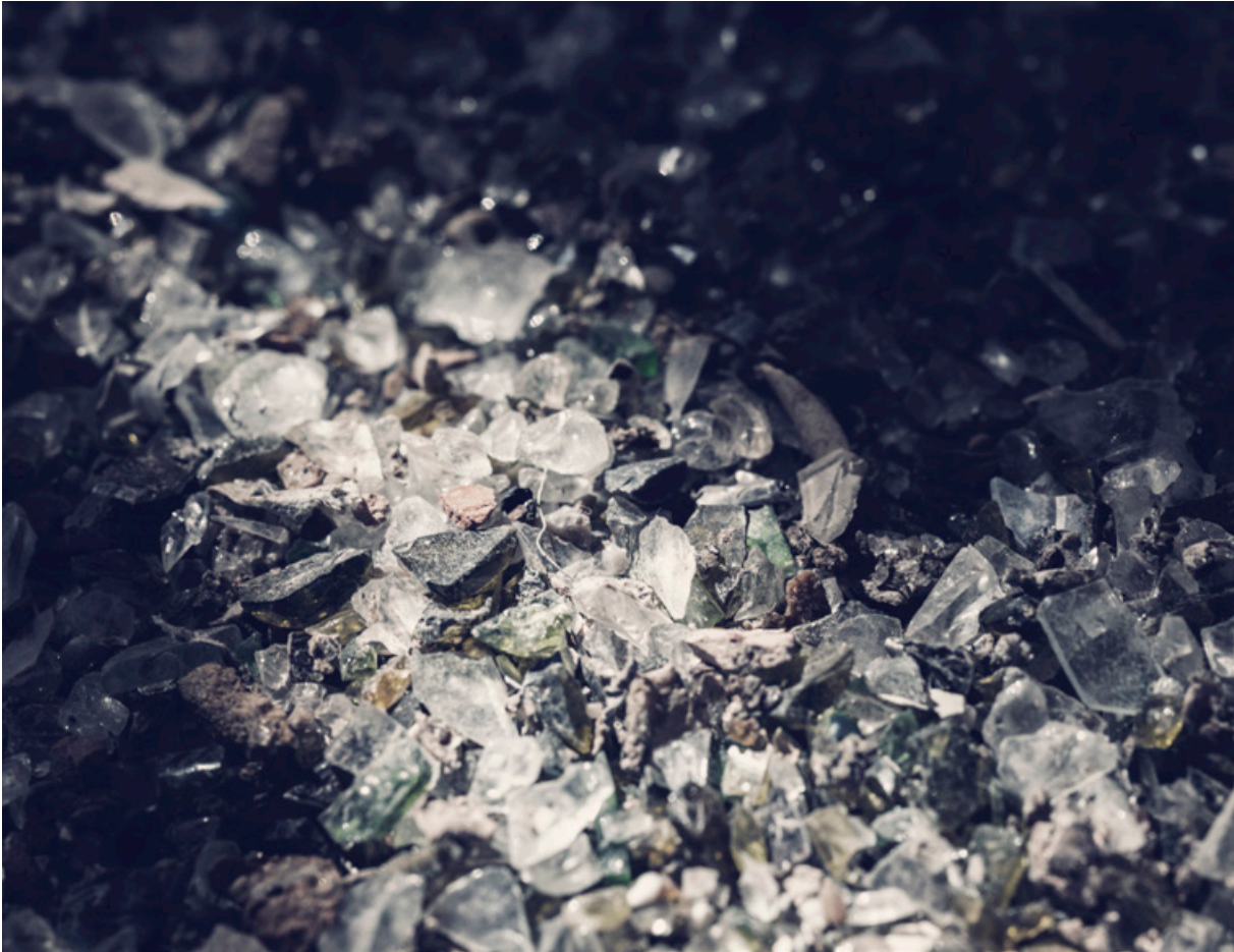
The reject consists of glass, gravel and sand.
